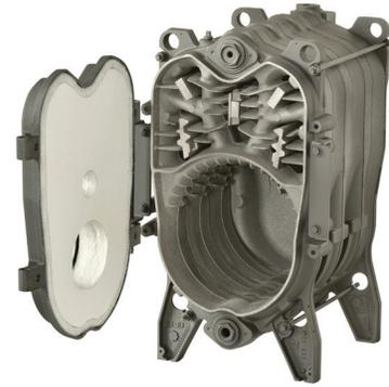
New DIAMOND Shape Sections help guide the flue gasses up the back wall and deflect them back towards the boiler door before it pushes back through the upper chamber to exit through the flue allowing more surface area for heat to transfer into the system water.
