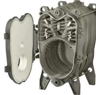
New DIAMOND-shaped sections direct flue gases up the rear wall, then back toward the boiler door before exiting through the upper chamber—maximizing heat transfer surface area and improving efficiency.
